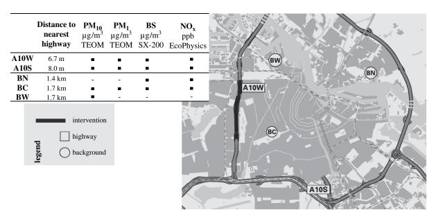
Fig. 1. Location of the speed limit intervention road section, the monitoring stations in Amsterdam Air Quality Monitoring Network, and monitored components.
